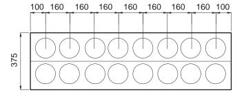
If ventilation ducts of 150 mm or larger are used in pairs, the initial and axial dimensions will change.
